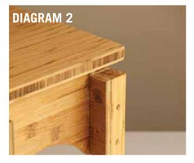
When attaching the legs, make sure that each leg is aligned with the side. Another tip is to hammer 2 dowels (instead of 4) only halfway in on each leg first to really help you line up the holes.
